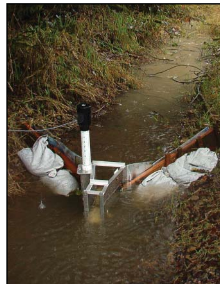
Flume and capacitance rod measuring ditch flows at Delwood Mainline site 2
